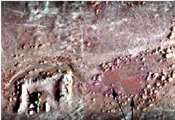
Camouflaged targets visually "disappear" into background. Visible region insufficient to positively discern camouflaged target(s)
