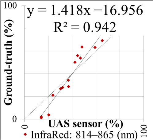
UAS imagery corresponding to OLI sensor bands, sensed by L8 overpass correlated with field spectroscopy measurements over EVA panels
