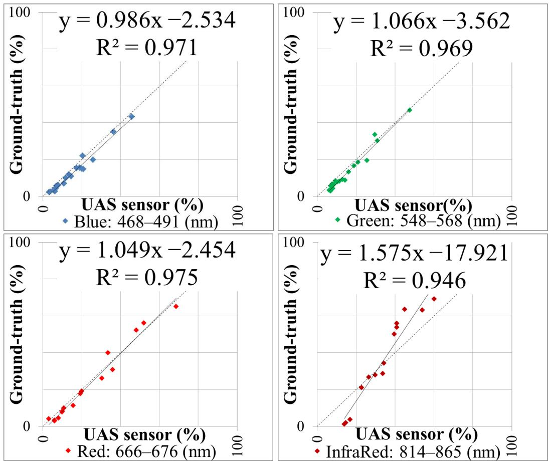
UAS imagery corresponding to MSI sensor bands, sensed by S2 overpass correlated with field spectroscopy measurements over EVA panels
