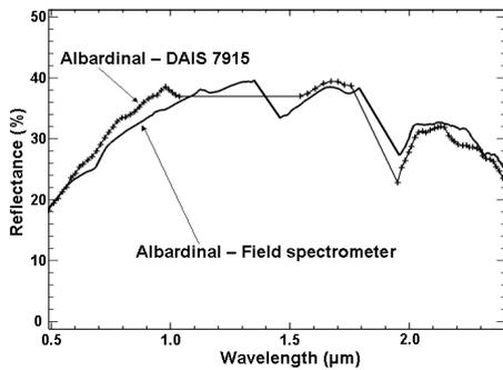
**Figure 6.-** Spectral characteristics of steppe vegetation (Albardinal) from the *anthropogenic affected floodplain* obtained with a Field spectrometer and DAIS 7915.
