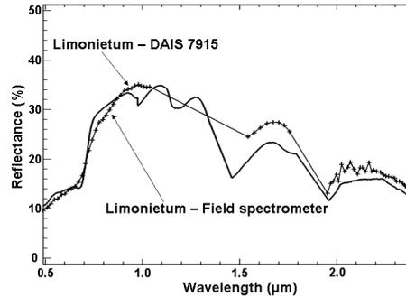
**Figure 7.-** Spectral characteristics of steppe vegetation (Limonietum) from the *anthropogenic affected floodplain* obtained with a Field spectrometer and DAIS 7915.
