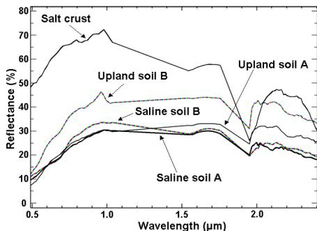
Figure 3.- Spectral characteristics of soils obtained with DAIS 7915.
