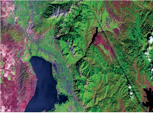
Figure 3. Image Pre-processing using ERDAS Imagine software: All seven bands (files, TIFF files) were downloaded and collapsed to form a single file (img format) using the “layer stack” function. Picture shows a Subset of the 2011-September Landsat image after it has been atmospherically corrected.
