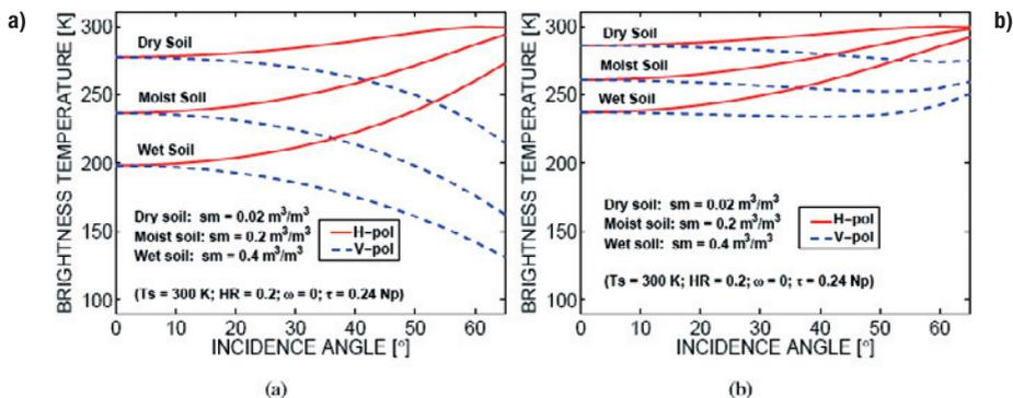
**Figure 2.** Brightness temperature dependence with incidence angle and polarization for (a) bare soil and (b) vegetation-covered soil.
