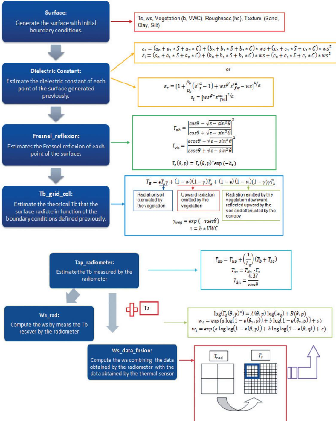
Figure 3. Flow Chart of HUMID simulator.
