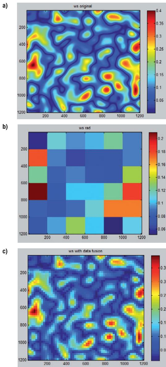
**Figure 4.** a) Initial soil moisture conditions for an arbitrary surface simulated, b) Soil moisture retrieved with the radiometer, c) Soil moisture by data fusion approach.
