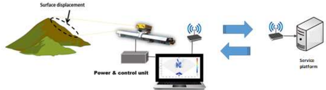
2) GBSAR discontinuous monitoring
