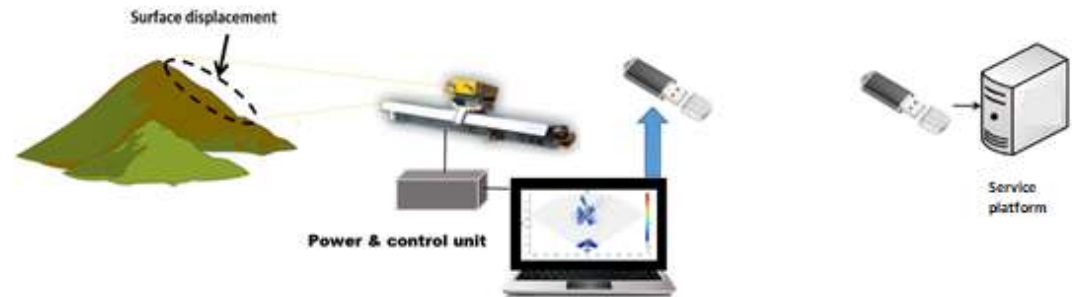
2) GBSAR discontinuous monitoring
